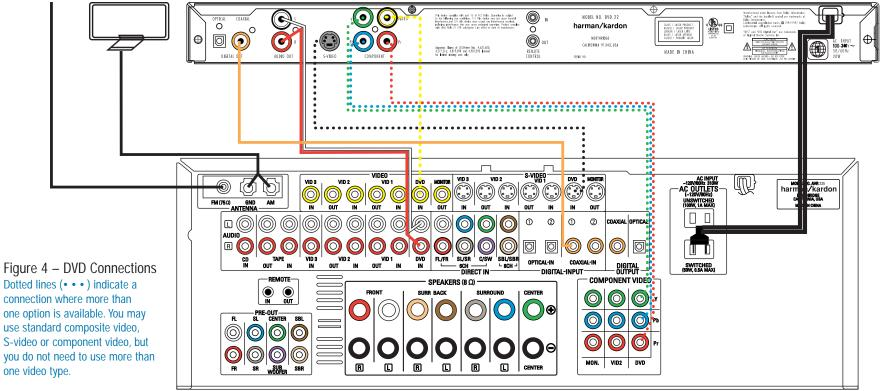
Step 4. Connect AM and FM antennas (as shown above). (See page 14.) Step 5. Connect the DVD 22 to the AVR 235 as shown above:
